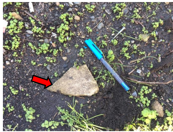
Photo 16: Suspected asbestos fragment on the exposed fill at 94 Carrington Road
