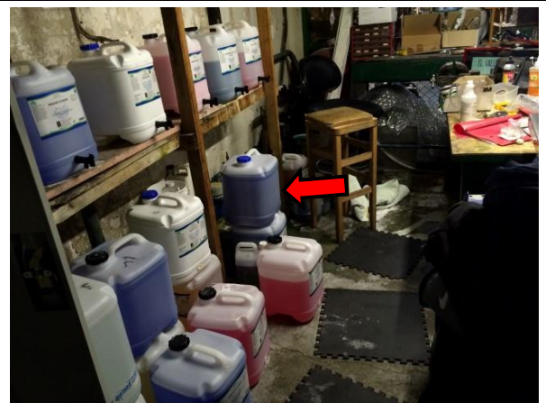
Photo 12: Cleaning chemicals stored without secondary containment in close proximity to a drain in the floor
