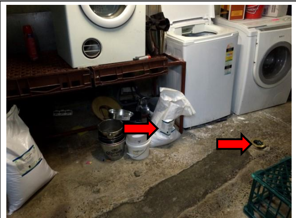
Photo 14: Washing chemicals stored without secondary containment in close proximity to a drain in the floor
